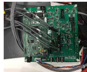
Laboratory prototype of the inverter and the controller
